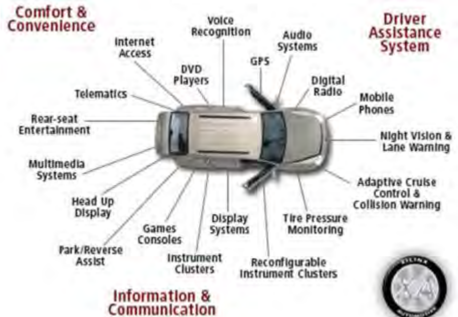
Automobile with multiple embedded systems.
