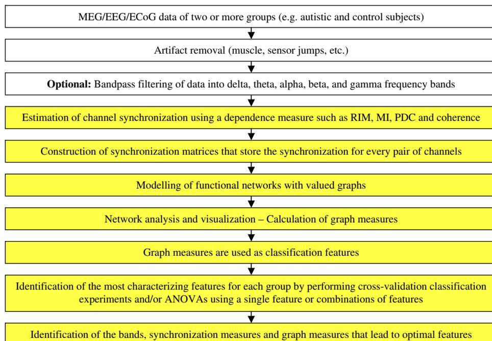
**Fig. 1.** Outline of the proposed methodology. In this paper we focus on steps represented by rectangles highlighted in yellow (steps 4–10). (For interpretation of the references to color in this figure legend, the reader is referred to the web version of this article.)
